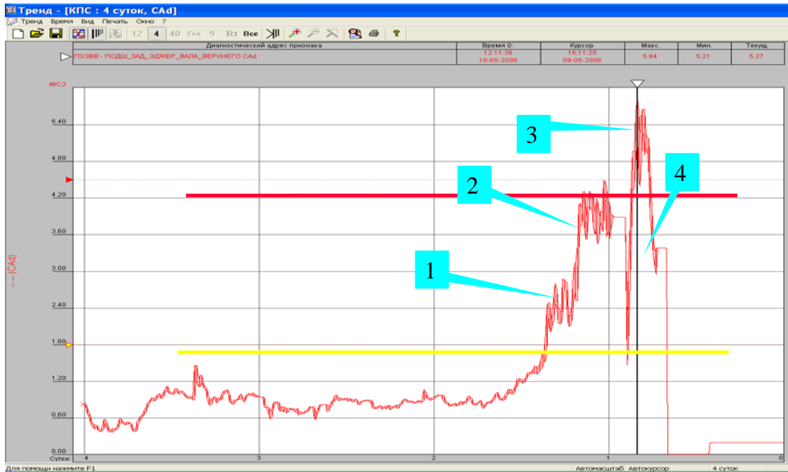
Figure 5. The trend of a multimodal exponential destruction (cut) of the wheel-rolling mill edging shaft: Sections 1-3 – multistage destruction of an upper edging shaft; Section 4 – the mill repair according to the actual technical state
