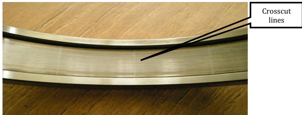
d) Inner surface of the outer ring of electric motor tail bearing
