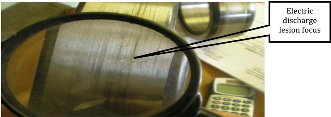
b) Electric discharge lesion focus on the outside surface of outer ring
