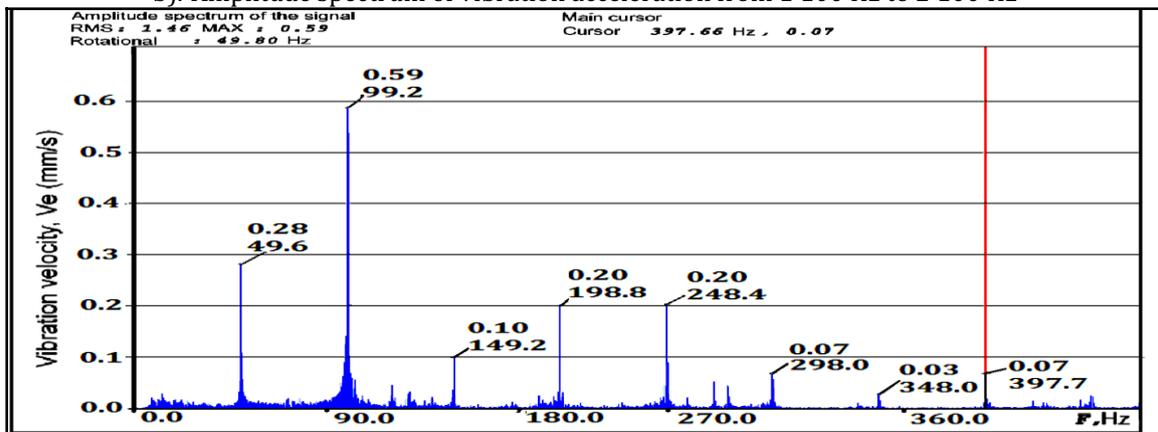
c). Amplitude spectrum of vibration velocity from 0 Hz to 450 Hz
