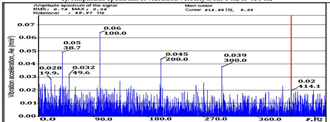
d). Envelope spectrum of a vibration acceleration signal from 0 Hz to 450 Hz
