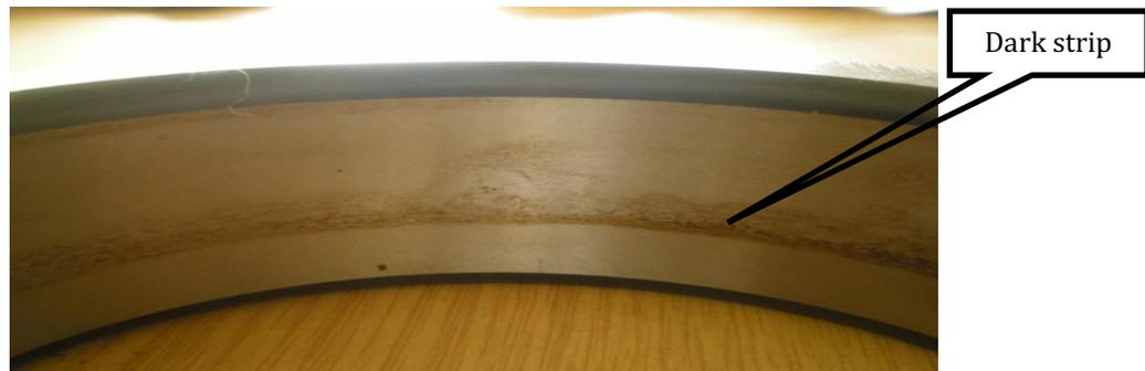
c) Inner surface of the cone of electric motor tail bearing
