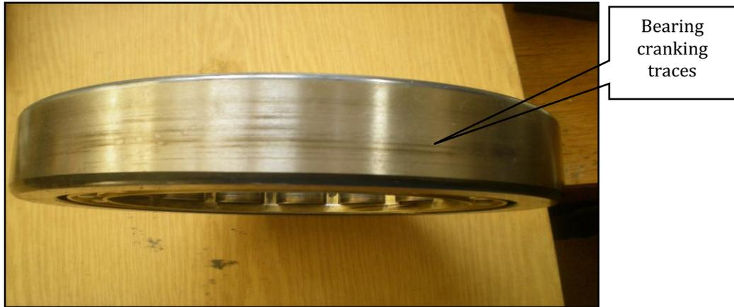
a) Outside surface of outer ring of electric motor tail bearing
