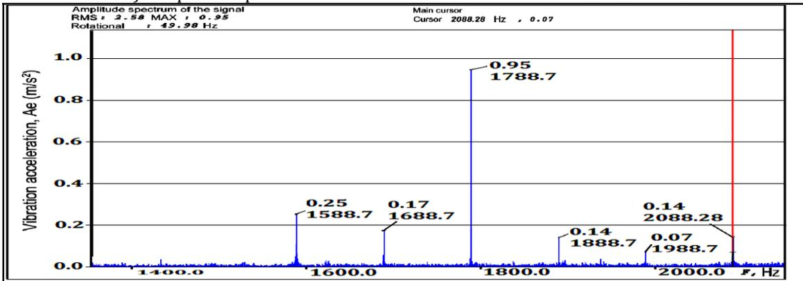
b). Amplitude spectrum of vibration acceleration from 1 100 Hz to 2 100 Hz
